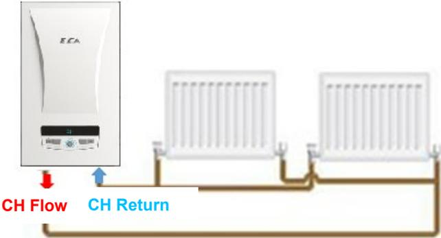
Figure 8. CH Device Installation Scheme
